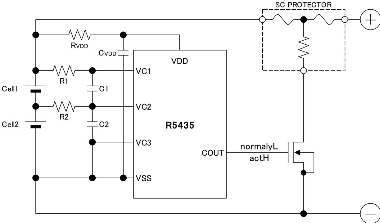
\*In terms of the order of connecting cells, the positive terminal of the cell 1 should be the last. Otherwise, COUT may output "H" tentatively, and the fuse may be fused.
