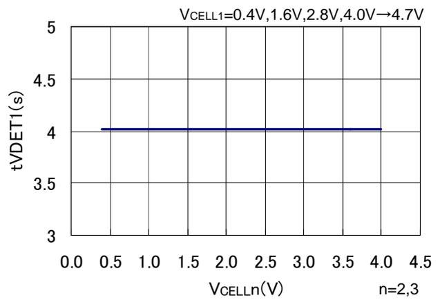
2) Output Delay of Release from Over-charge vs.  $V_{DD}$
