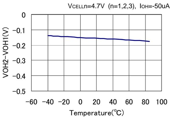
9) C<sub>OUT</sub> Nch ON Voltage vs. Temperature
