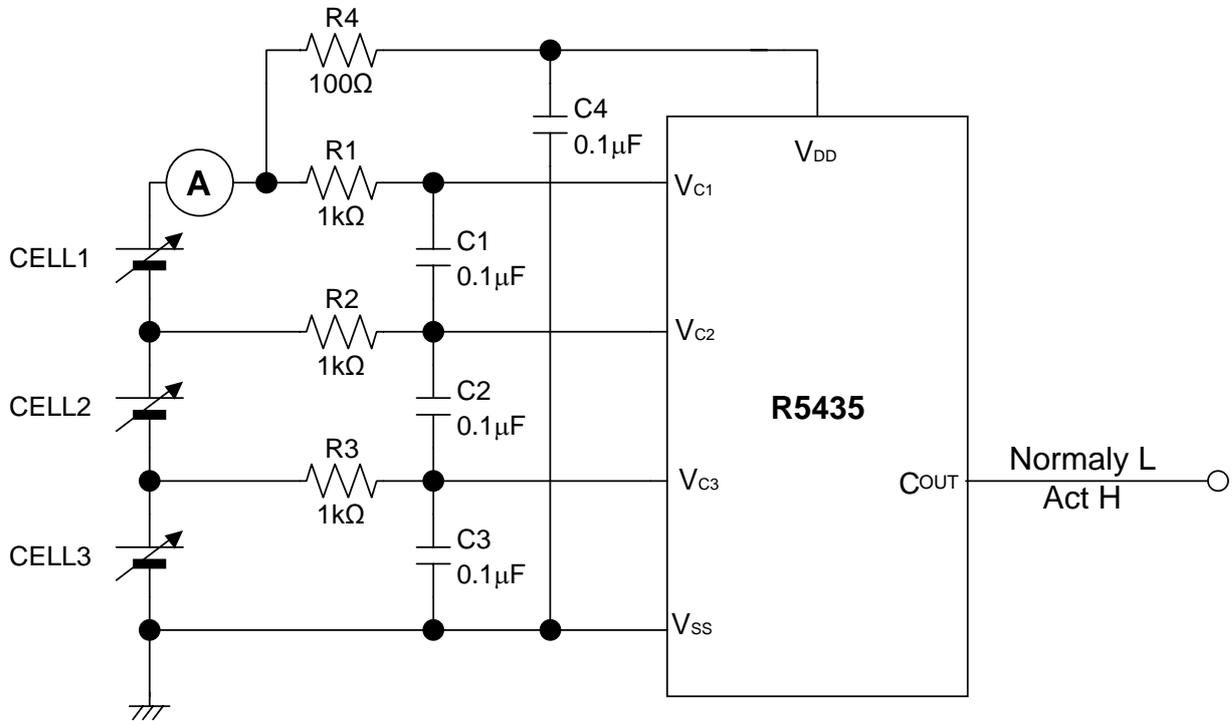
**3-cell protector Supply Current vs.  $V_{DD}$**
