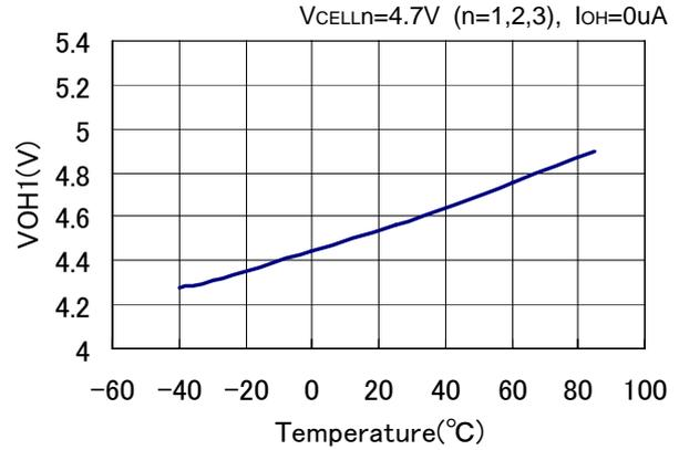
8) C<sub>OUT</sub> Pch ON Voltage 2 vs. Temperature
