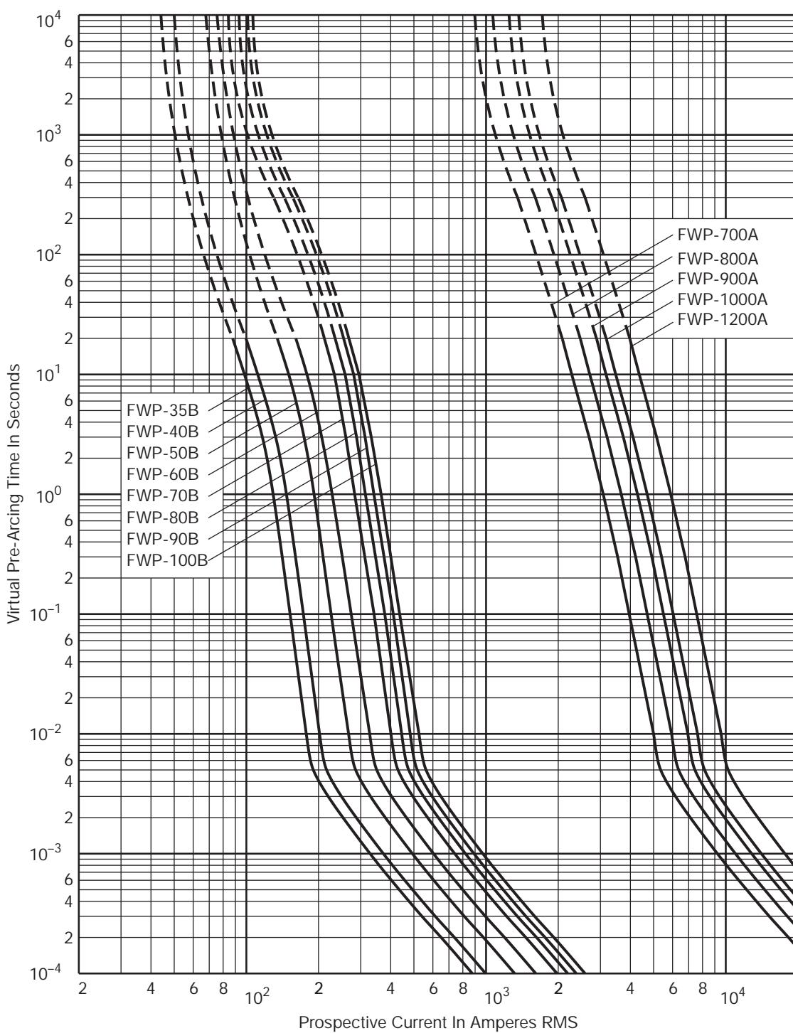
**Minimum Melting** Time-Current Characteristic Curves
