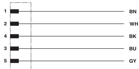
Contact assignment of the M12 plug
