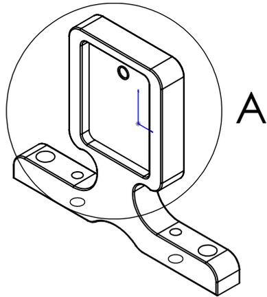
Use the 1/2" #6-32 screws with the outer unthreaded mounting holes, using a 7/64 hex key. Sized for Arlo Base Kit.
