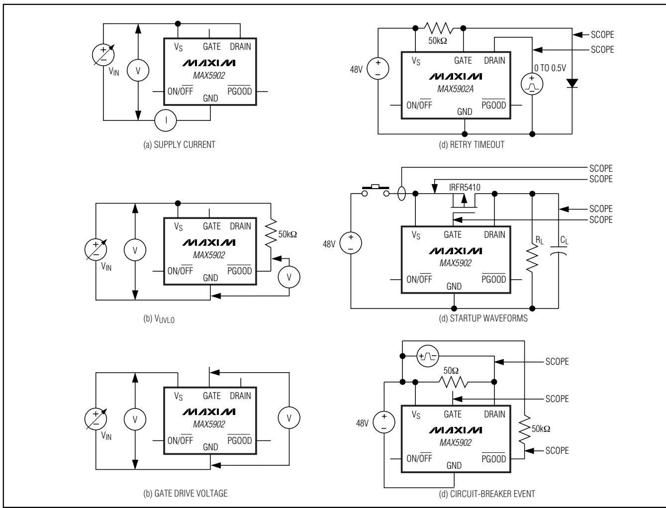
Figure 2. Test Circuits
