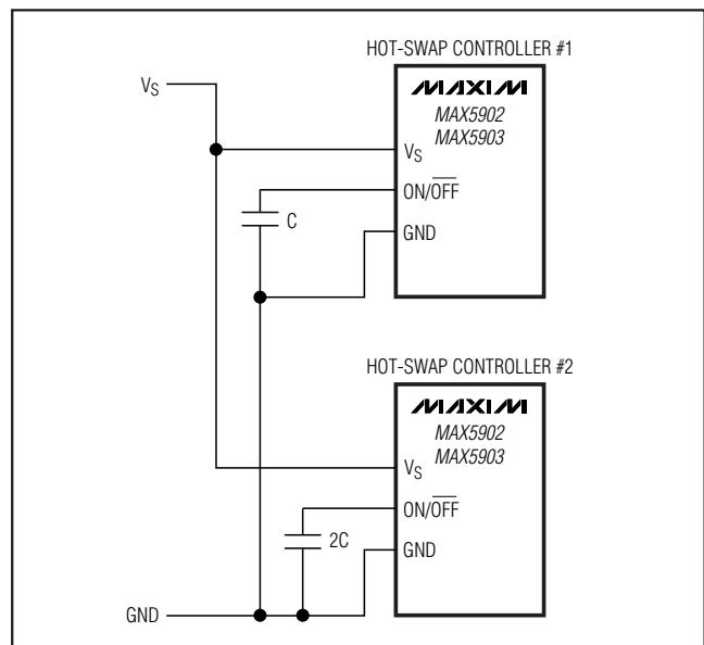
Figure 4. Power-Supply Sequencing
