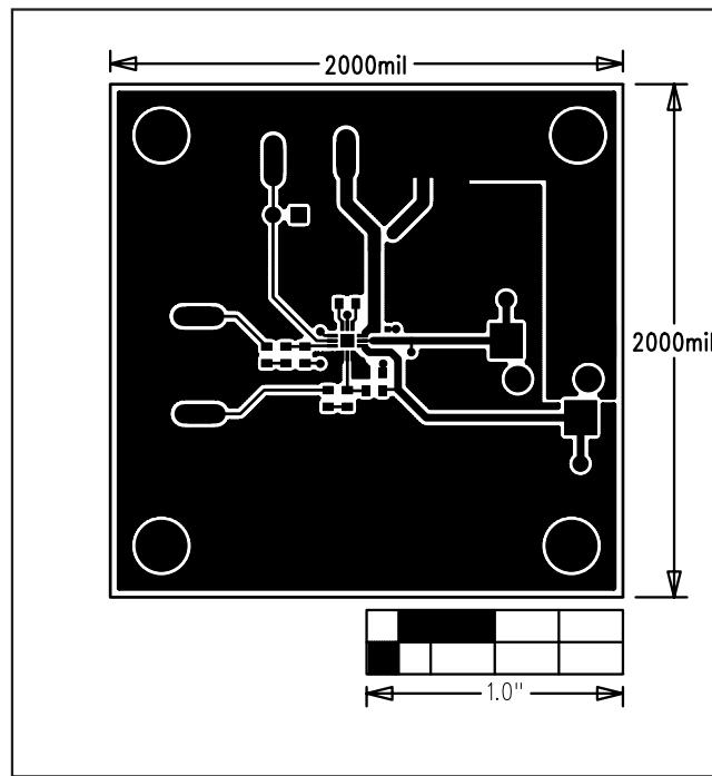
Figure 3. MAX9724A EV Kit PCB Layout—Component Side
