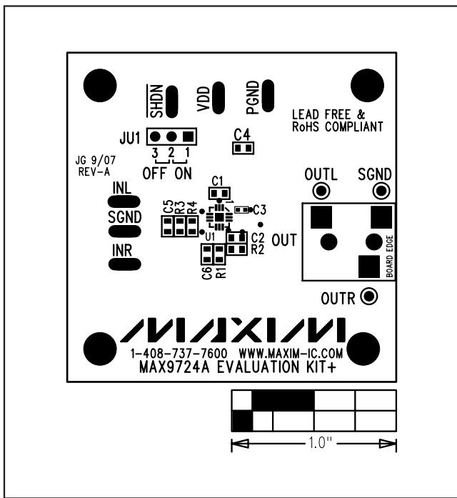
Figure 2. MAX9724A EV Kit Component Placement Guide—Component Side
