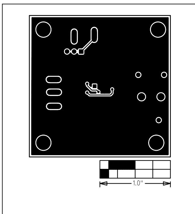
Figure 4. MAX9724A EV Kit PCB Layout—Solder Side
