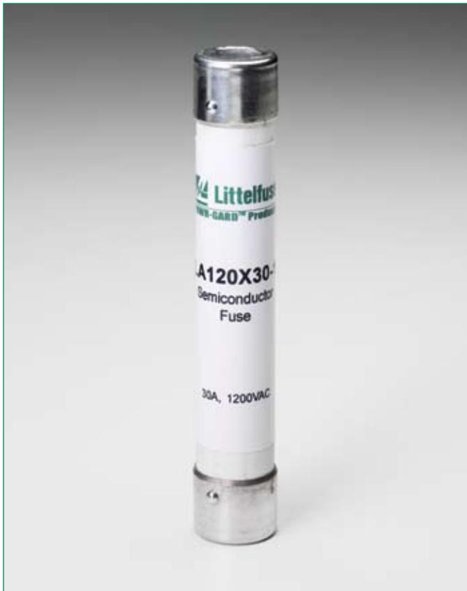
Littelfuse LA120X semiconductor protection fuses, rated 1/2 through 30A, 1200 VAC are popular for use in traction drive auxiliary circuits and similar applications. LA120X fuses are also suitable for use on 1000VDC auxiliary circuits with low time constants.
