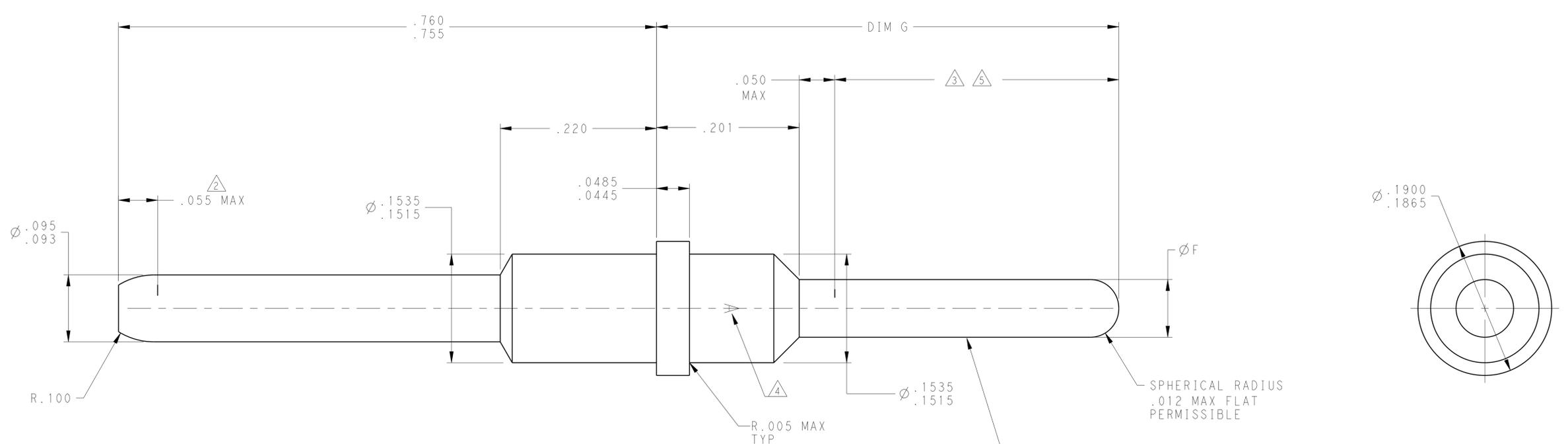
MAT'L: COPPER ALLOY PER ASTM-B-301
