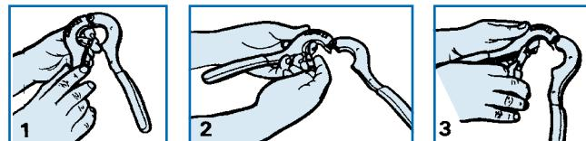
**Replacing Insert Pads in Backshell Assembly Tools**
