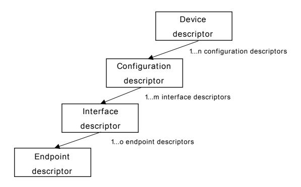
As can be seen, the descriptors form a tree. The root is the device descriptor with n configuration descriptors as children, each of which has m interface descriptors which in turn have o endpoint descriptors each.
