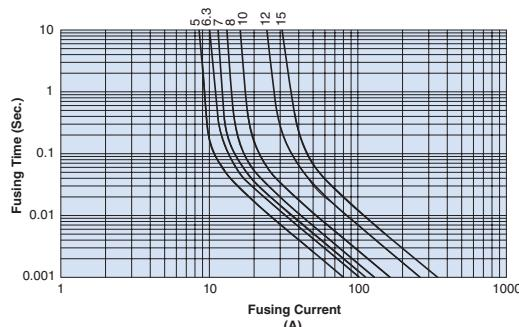
Stationary Current: Regard the peak of stationary current waveform as stationary current value when the stationary current is repeated pulse. Normal derating of this product should be 0.7max. as standards.
