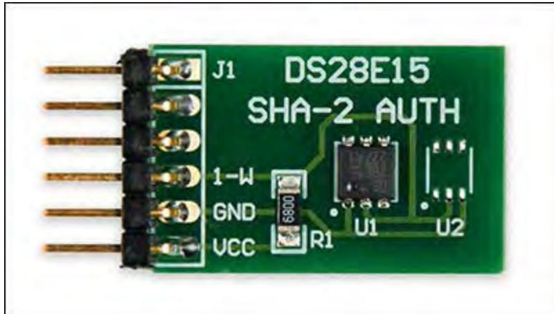
implement SHA-256 authentication on Xilinx® FPGAs. The DS28E15 communicates over the single-contact 1-Wire® bus, reducing the number of pins necessary to carry out the solution. The reference code defines a combined SHA-256 processor and 1-Wire Master on the host FPGA.
