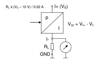
R<sub>L</sub> range depending on V<sub>S</sub> for proper operation
