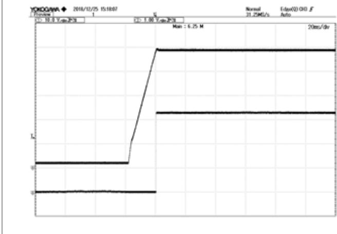
Figure 9: PG voltage vs. Vout @ Vin=220Vac, 0A lout TOP: Vout, 10V/div, 20mS/div BOTTOM: PG, 1V/div, 20mS/div
