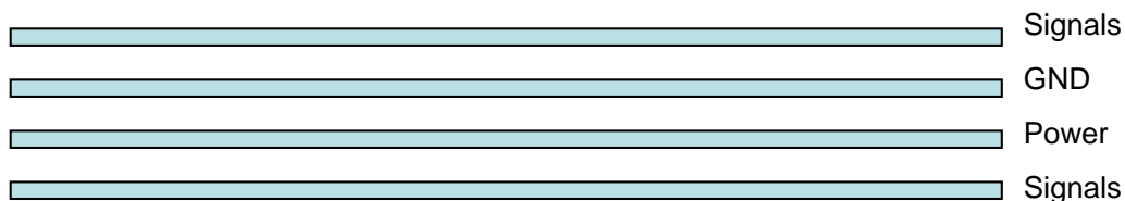
Figure 29: Typical 4-layer PCB construction
