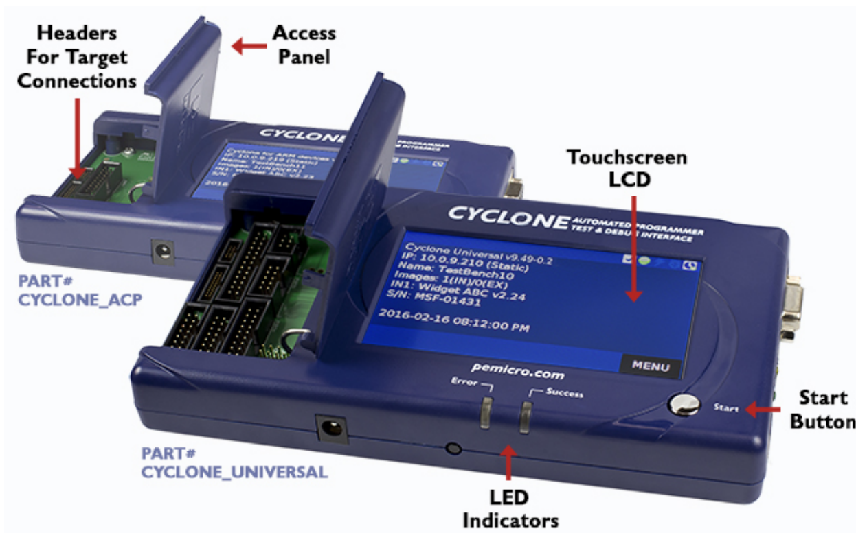
Figure 3-1: Cyclone LC Top View
