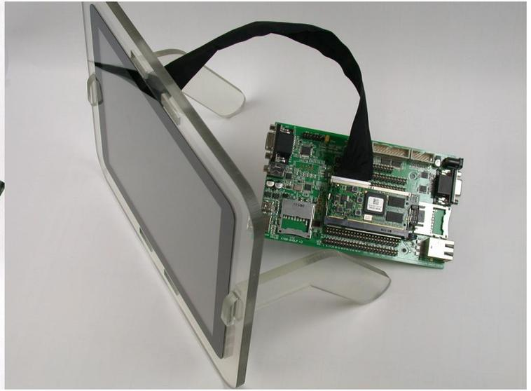
This two piece adapter supports the direct connection of Freescale's 10.1" 1024x768 (XGA) display with capacitive touch (Freescale part no.: MCIMX-LVDS1 / not included)
