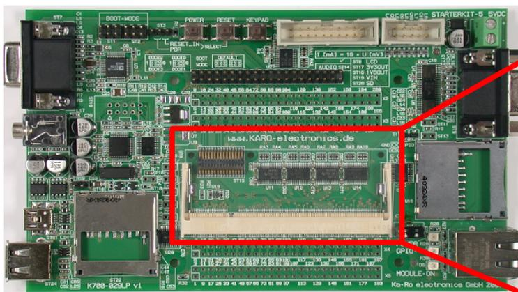
The second part is mounted on top plugged into the two 100-pin connectors:
