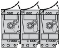
Remove the protective cover from the top of the drive.
