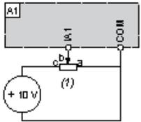
(1) 2.2 k $\Omega$ ...10 k $\Omega$  reference potentiometer
