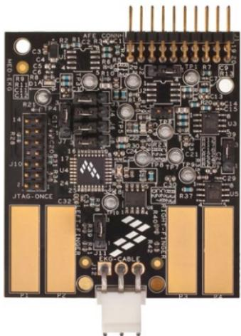
Figure 4: MED-EKG with Default Jumpers Used in Table 2
