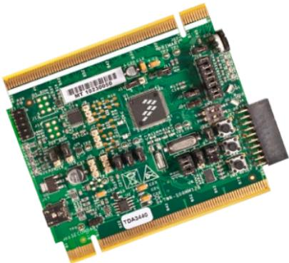
**Figure 3: TWR-S08MM128 with Default Jumpers
