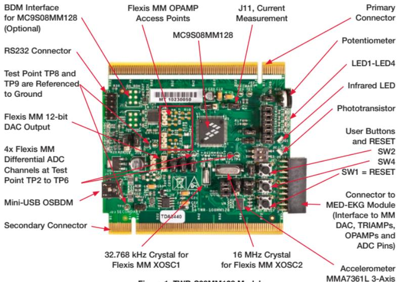
Figure 1: TWR-S08MM128 Module
