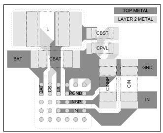
Figure 4. Power PCB Layout Example
