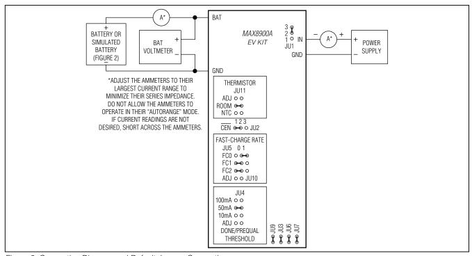
Figure 3. Connection Diagram and Default Jumper Connections
