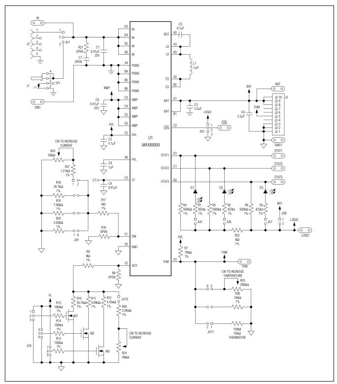
Figure 9. MAX8900A EV Kit Schematic
