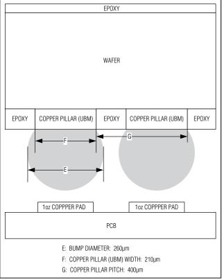
Figure 6. Bump Cross Section and Copper Pillar Detail
