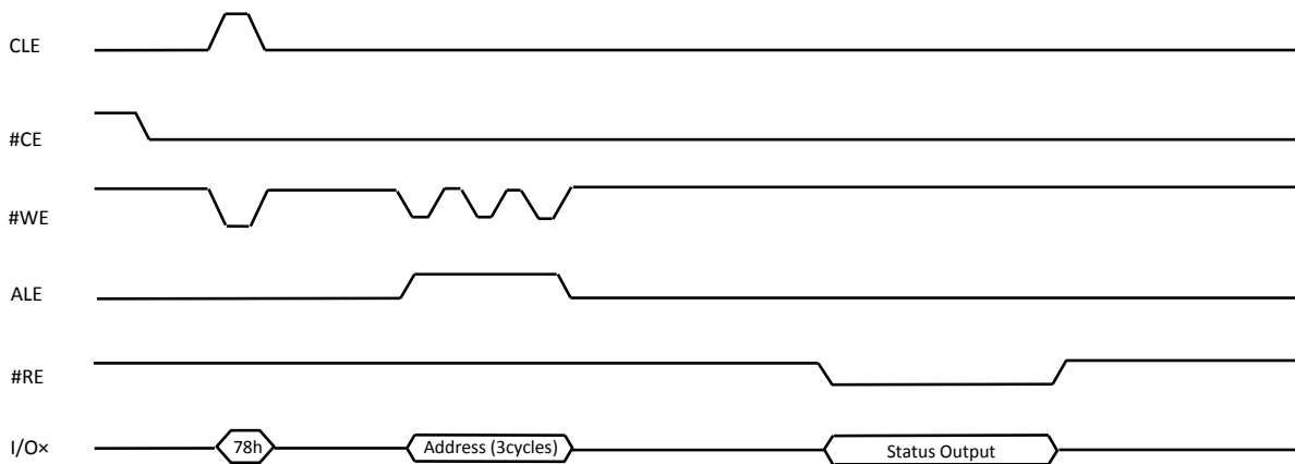
Figure 9-10 Read Status Enhanced (78h) Operation
