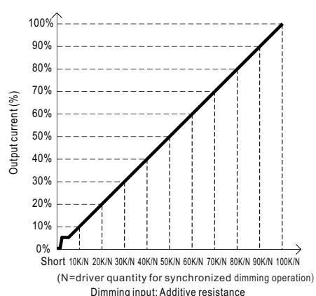
Note : 1. Min. dimming level is about 8% and the output current is not defined when 0% < Iout < 8%.
