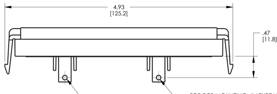
FOR PCB MOUNTING, #4 THREAD CUTTING SCREWS (TYPE 23 OR SIMILAR) ARE RECOMMENDED; TORQUE TO 2-3 IN\*LBS [0.23-0.34Nm]
