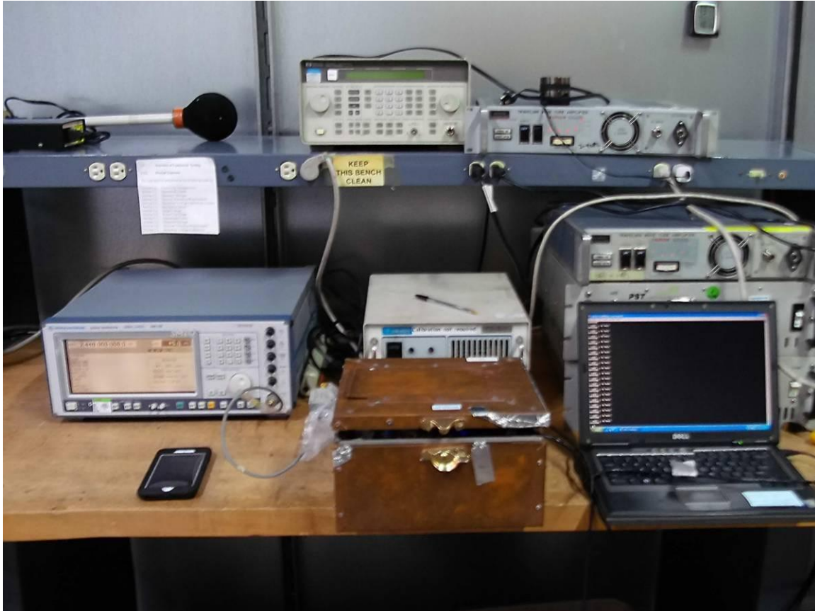
Figure 37. Receiver Blocking Test Setup
