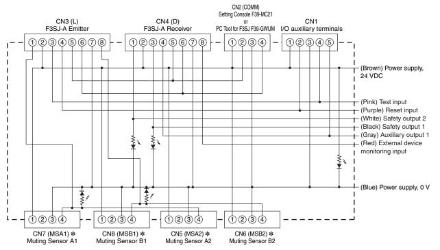
\* Use the following connecting cable to connect the Muting Sensors:
