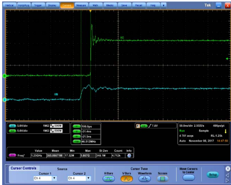
Figure 32. High Side Turn-Off Propagation Delay (NCP51530B)
