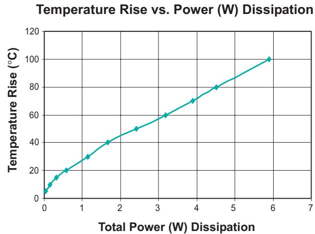
$$\text{Total Power Dissipation} = \text{Copper Loss (W)} + \text{Core Loss (W)}$$
