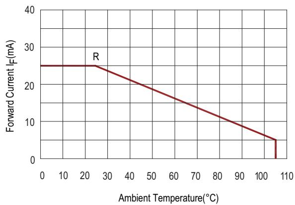
**Figure 3. Allowable DC Current vs. Ambient Temperature**
