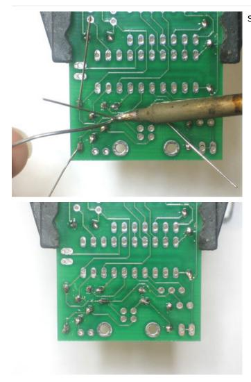
Solder and clip the diode leads.
