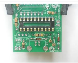
Next is the socket for the microcontroller that does all the hard work. A socket is useful because you can replace the chip in case of upgrade or damage. Sockets have a little notch in them to indicate which way to put in the chip. This notch should match the notch in the silkscreen image, in this picture, the notch is on the lefthand side.
