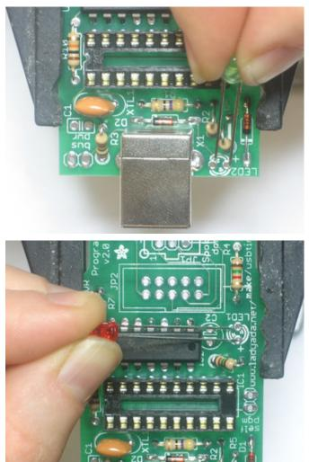
Next are the two indicator LEDs, green **LED2** and red **LED1**. These LEDs let you know that the USB device connected successfully, and is in the process of programming the target device.
