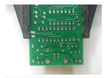
When you are done, it should look like this. If you have some sticky stuff on the solder joints, that's OK, that's the rosin inside the solder that protects the joints from oxidation. It isn't necessary to clean it off.
