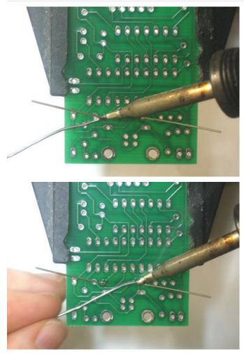
Next, with your soldering iron, solder each of the resistor legs. Place the tip of the iron against both the pad (ring) and lead (leg) and after a few counts, touch the solder in, to make a nice joint.
