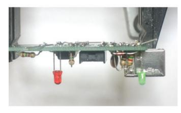
The LEDs are also supposed to be very close to the top of the enclosure, so that you can see the light through the drilled holes, when you bend the leads, make sure the LEDs stick out about 1/2" above the PCB.
