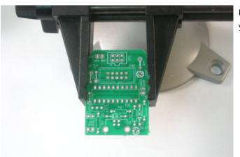
Put the PCB in the vise & heat up the soldering iron so you are ready to go!
