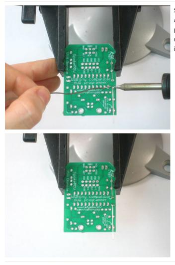
Solder the legs. Hold the tip of iron against the wire leg and the metal ring at the same time, after 2 counts, poke the solder in till it creates a nice pool. Then remove the solder, wait a half count, then remove the iron. Do this for both legs.
