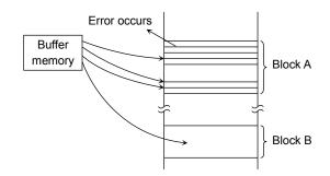
When an error happens in Block A, try to reprogram the data into another Block (Block B) by loading from an external buffer. Then, prevent further system accesses to Block A (by creating a bad block table or by using another appropriate scheme).
