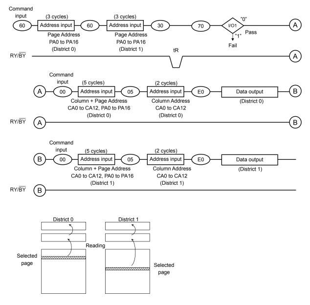
The data transfer operation from the cell array to the Data Cache via Page Buffer starts on the rising edge of  $\overline{\text{WE}}$  in the 30h command input cycle (after the 2 Districts address information has been latched). The device will be in the Busy state during this transfer period.
