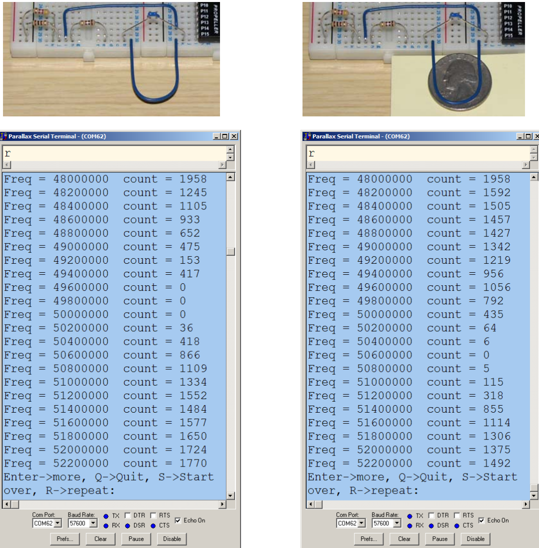
Figure 7-31: Calibrated Metal Detector Response – without metal (left) and with metal (right)
