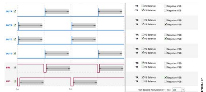
Figure 65. Volt-Second Balance with Register 0xFE56 = 0x69
