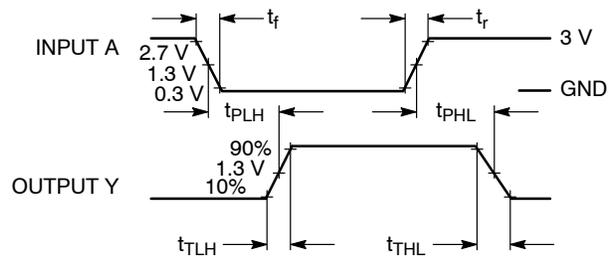
**Figure 1. Switching Waveforms**
