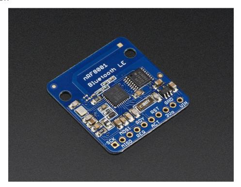
Our nRF8001 Breakout allows you to establish an easy to use wireless link between your Arduino and any compatible iOS or Android (4.3+) device. It works by simulating a UART device beneath the surface, sending ASCII data back and forth between the devices, letting you decide what data to send and what to do with it on either end of the connection.
