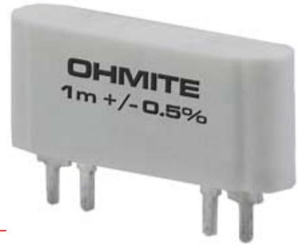
The CS5 is a high power precision current sensing resistor designed with four terminals. This resistor series is distinguished by excellent long term stability & TCR. The Kelvin connections allow high precision measurements even with low resistance values. The CS5 series has a non-inductive copper manganin element inserted into a cement sealed ceramic case.
