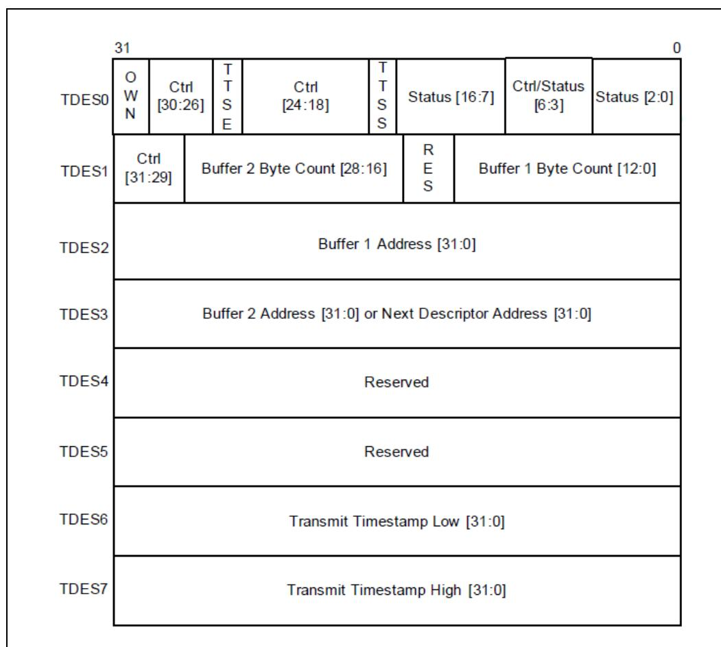
The DMA always reads or fetches four DWORDS of the descriptor from system memory to obtain the buffer and control information as shown in [Figure 30](#). When the AV feature is enabled, TDES0 has additional control bits[6:3] for Channel 1 and Channel 2. For Channel 0, Bits [6:3] are ignored. Bits [6:3] are described in [Table 89](#).
