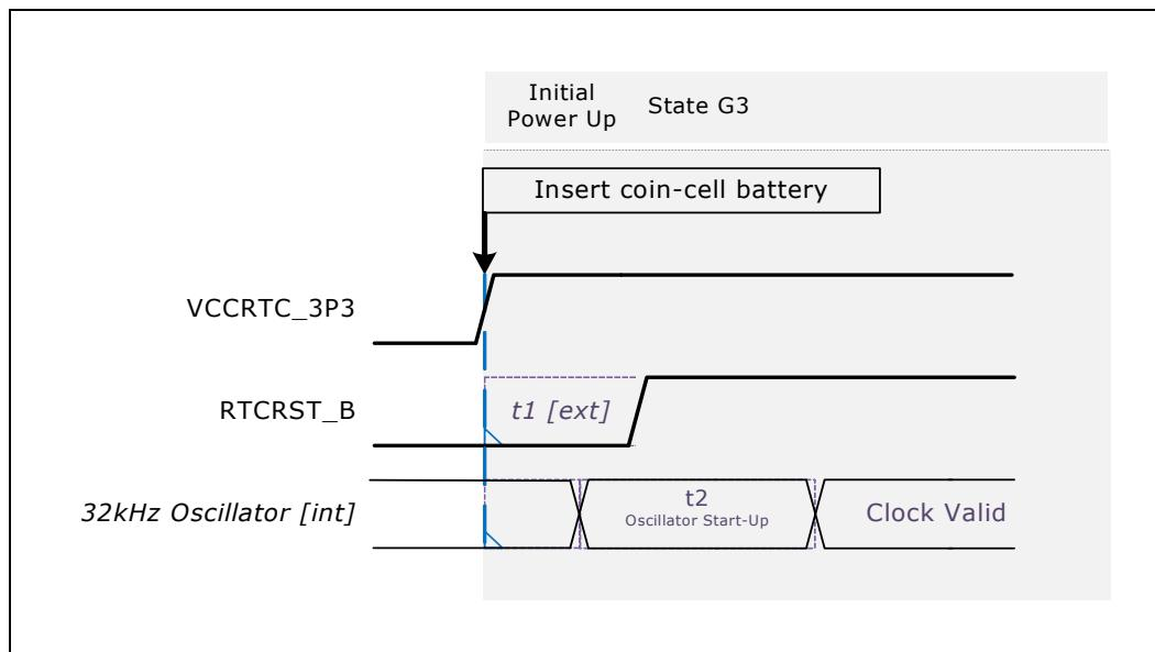
**Table 66.** RTC Power Well Timing Parameters
