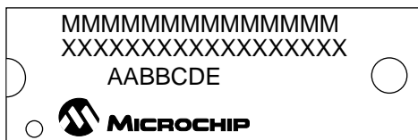
40-Lead CERDIP Windowed
