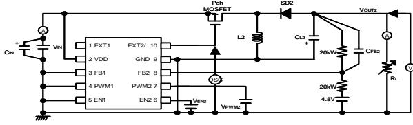
■ External Components of the Test Circuits
