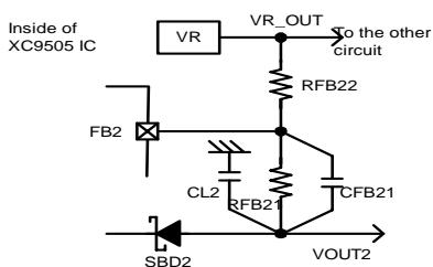
A stable positive voltage produced by a positive-voltage regulator or by other means is usable.
