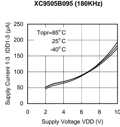
(13) Supply Current 1-4 vs. Supply Voltage
