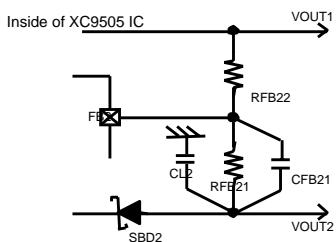
Channel 1 (Step-Down) circuits should be enable by setting EN1 to High level so that a stable voltage is provided. Inrush current to the inverter when the supply voltage VDD of the IC is 2.0 V or higher can be controlled by setting EN 1 and EN 2 to enable ("H" level) simultaneously.
