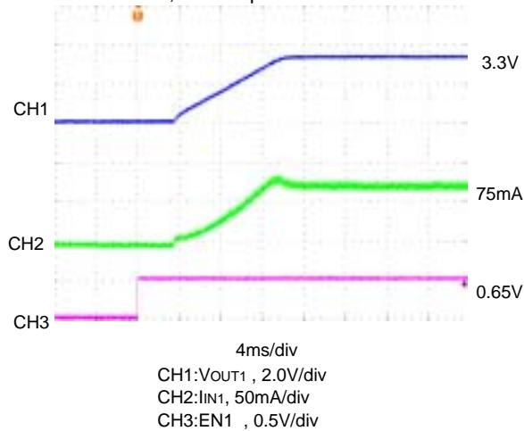
&lt; 2 ch. Inverting DC/DC Controller &gt;
