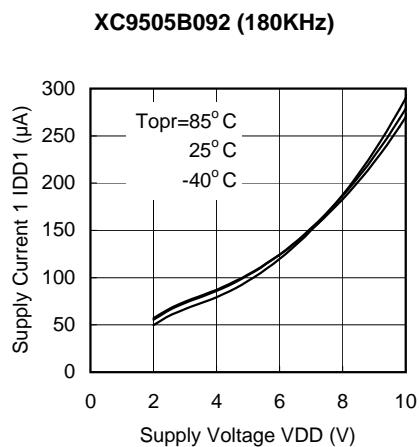
(10) Supply Current 1-1 vs. Supply Voltage
