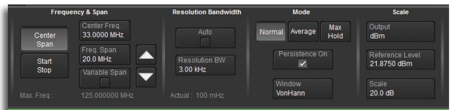
Spectrum analyzer style controls simplify waveform analysis in the frequency domain.
