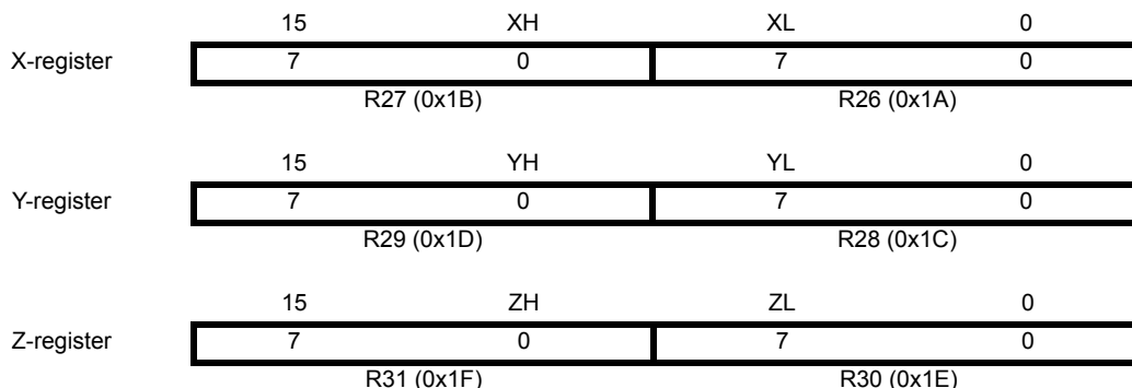
Figure 4-4. The X-, Y-, and Z-registers
