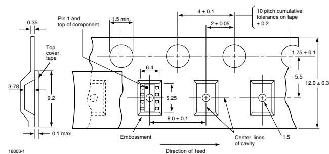
Fig. 9 - Tape Dimensions, 2000 Parts per Reel
