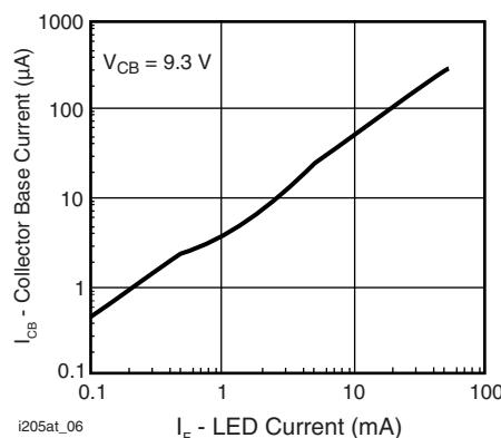
Fig. 7 - Collector Base Photocurrent vs. LED Current
