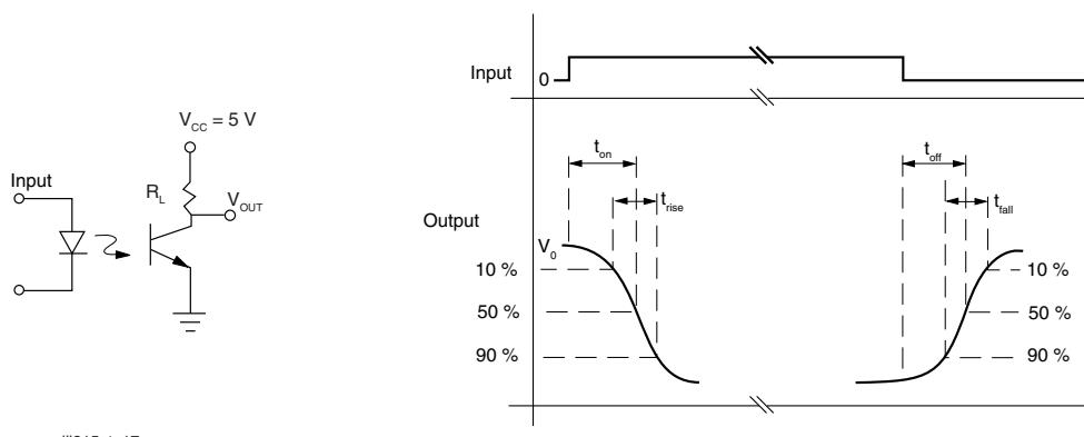
**Fig. 1** Switching Test Circuit
