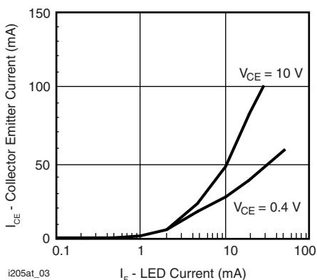
Fig. 4 - Collector Emitter Current vs. LED Current
