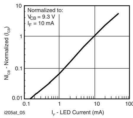
Fig. 6 - Normalized Collector-Base Photocurrent vs. LED Current
