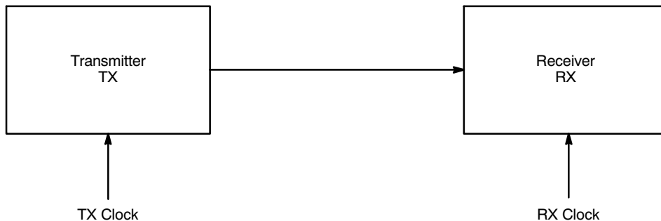
Figure 33. Example of a Serial Data Transmission System
