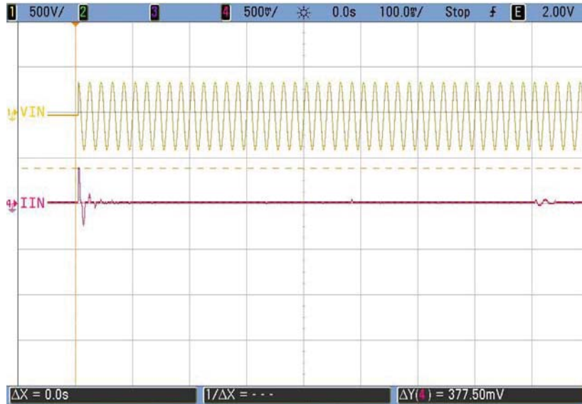
Time: 100 mSec/Div, Ch1: 500 V/Div, Ch4: 20 A/Div, Vin: 264 VAC, Ipk = 15.1 A AC applied at peak of sine wave
