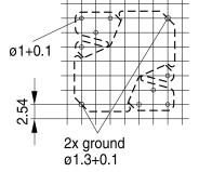
Hole arrangement View in mounting direction
