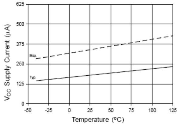
Figure 18A. V<sub>CC</sub> Supply Current vs. Temperature
