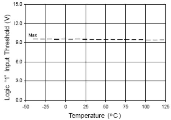
Figure 12A. Logic "1" Input Threshold vs. Temperature
