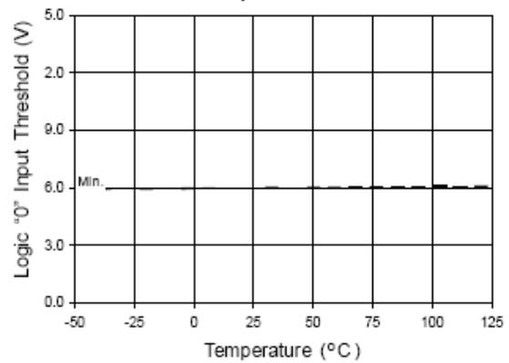
Figure 13A. Logic "0" Input Threshold vs. Temperature
