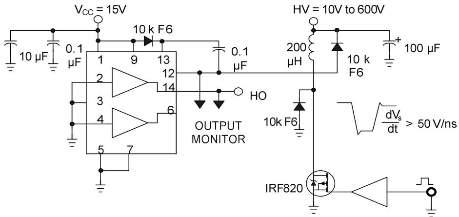
**Figure 2: Floating Supply Voltage Transient Test Circuit**
