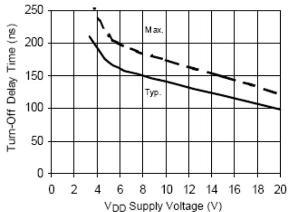
Figure 8C. Turn-Off Time vs. V<sub>DD</sub> Supply Voltage
