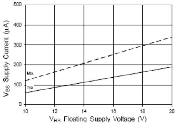
Figure 17B. V<sub>BS</sub> Supply Current vs. Voltage
