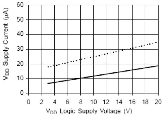
Figure 19B. V<sub>DD</sub> Supply Current vs. V<sub>DD</sub> Voltage
