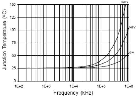
Figure 28. IRS2110/IRS2113 T<sub>J</sub> vs. Frequency (IRFBC20) R<sub>GATE</sub> = 33 Ω, V<sub>CC</sub> = 15 V
