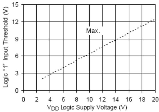
Figure 12B. Logic "1" Input Threshold vs. Voltage
