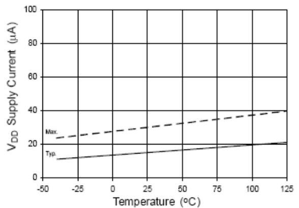
Figure 19A. V<sub>DD</sub> Supply Current vs. Temperature
