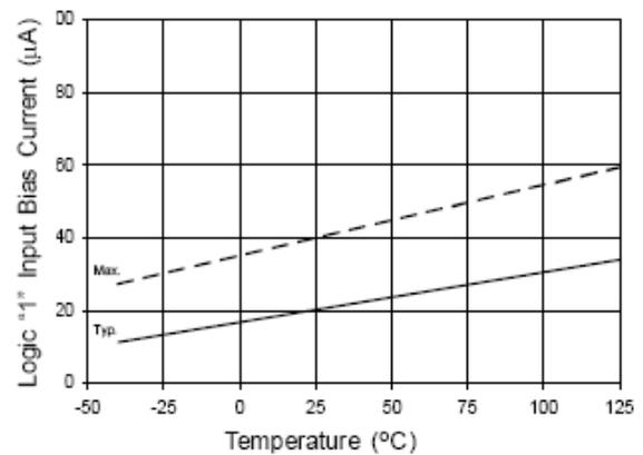
Figure 20A. Logic "1" Input Current vs. Temperature
