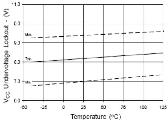
Figure 25. V<sub>CC</sub> Undervoltage (-) vs. Temperature
