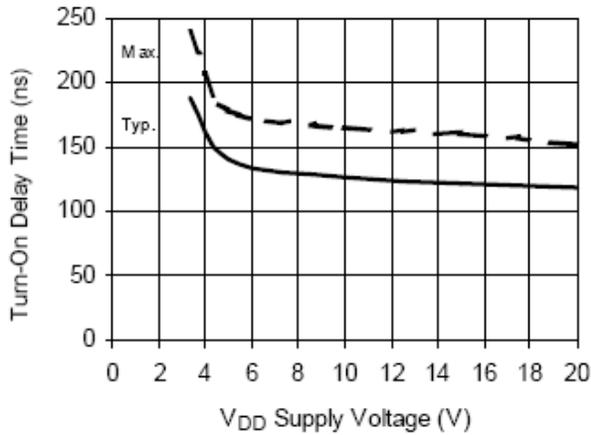
Figure 7C. Turn-On Time vs. V<sub>DD</sub> Supply Voltage
