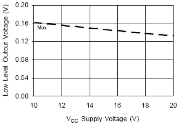
**Figure 15B. Low Level Output vs. Supply Voltage**
