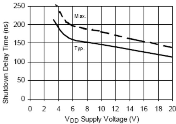
Figure 9C. Shutdown Time vs. VDD Supply Voltage
