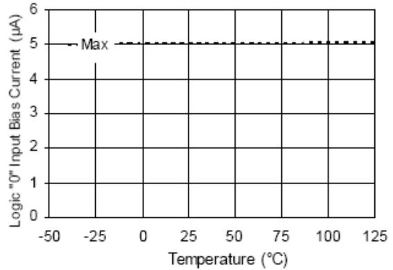
Figure 21A. Logic "0" Input Bias Current vs. Temperature
