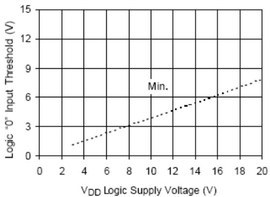
Figure 13B. Logic "0" Input Threshold vs. Voltage
