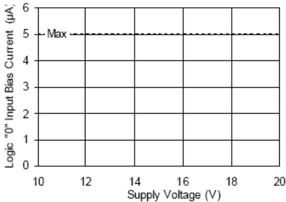
Figure 21B. Logic "0" Input Bias Current vs. Voltage
