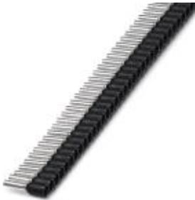
Taped ferrules, 1.5 mm<sup>2</sup>, sleeve length 8 mm, with plastic collar, according to DIN 46228-4, black, for processing with the CRIMPFOX 4 IN 1, 10 strips each with 50 sleeves per strip.
