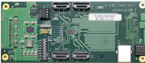
89KT0604S 2-lane, with I 2 C Configuration
