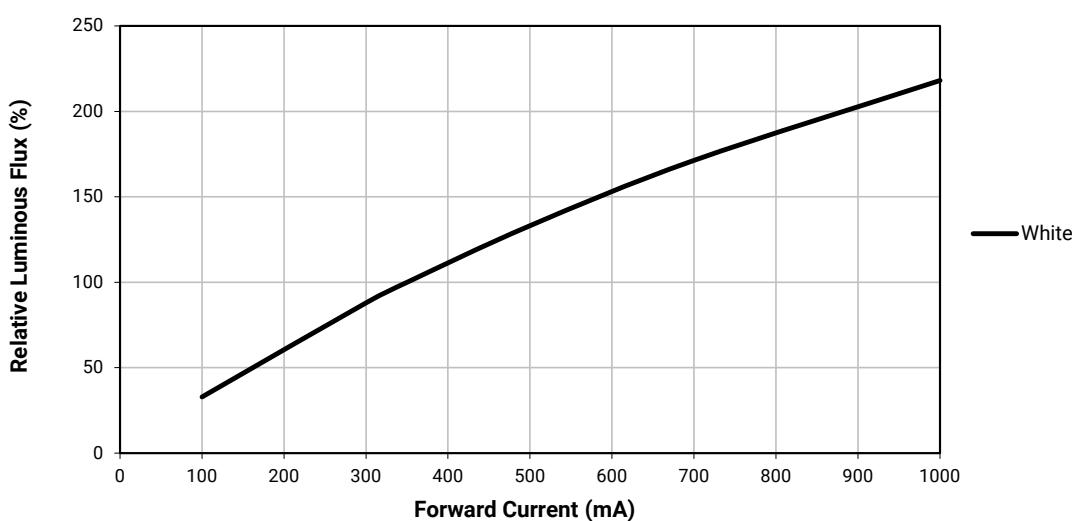
RELATIVE FLUX VS. CURRENT - COLOR ( $T_J = 25^\circ\text{C}$ )
