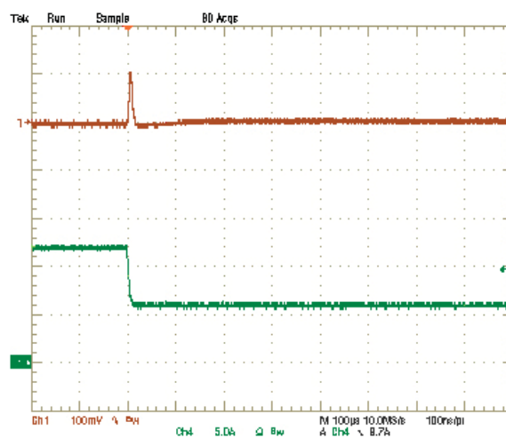
Step Load Transient Response (Vin=5.0V, Vout=3.3V, Cload=94μF, Iout=12A to 6A) Trace 1=Vout, 100 mV/div, Trace 4=Iout, 5A/div.
