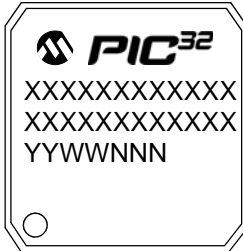
100-Lead TQFP (12x12x1 mm)
